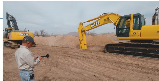
**Although recording sound levels at 50 feet with the machine actually working was not part of the recommended checking procedures, we were curious. On average, the 350D was about 6 dB(A) quieter.**
