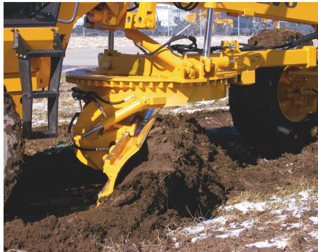
**The graders are designed with the transmission ahead of the articulation joint, an engineering feature that adds weight to the moldboard and enhances productivity, according to Volvo.**
