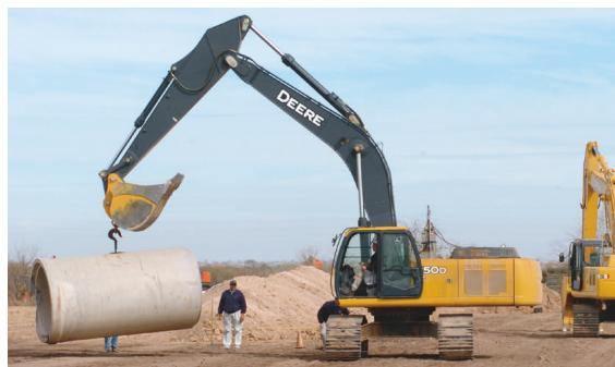
**In the over-side lifting exercise, operator Mike Boyle armed out until the rollers just lifted from the rails on the opposite track. We then measured the radius (center of the swing bearing to center of the lifting hook).**
