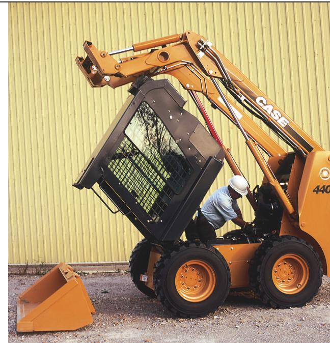
**The ROPS/cab on Case's 400 Series tilts in 10 seconds for open access to the engine and major hydrostatic components under the operator's compartment. Case 400 Series skid-steer loaders have a single location for all daily service checks.**
