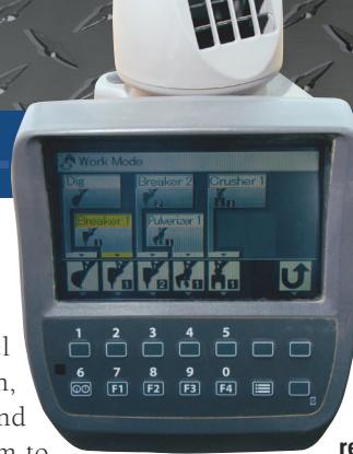
**The D-Series monitor has considerably more capability than that used in the C-Series. The user can employ the system for checking operating parameters, setting hydraulic requirements for multiple tools, tracking service intervals and for performing diagnostic investigation.**
