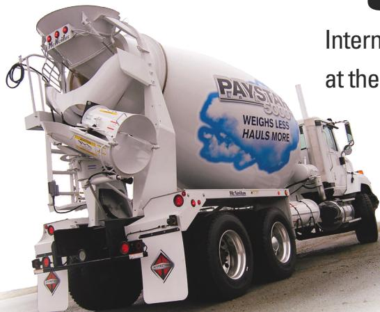
**The biggest weight cutter is the McNeilus Revolution body with its fiberglass drum. It saves 2,000 pounds compared to a steel drum.**
