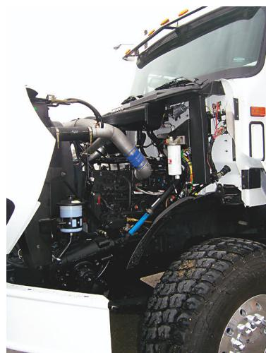
**The engine's not International's own DT 570, but a Cummins ISL. It's lightweight, but makes hefty power and torque.**
