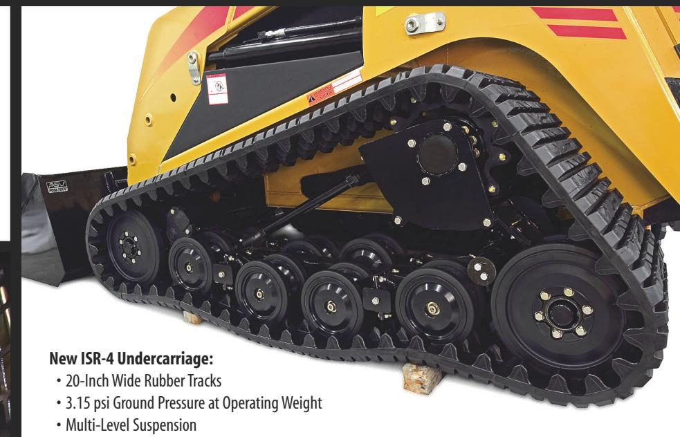
**THE NEW Posi-TRACK SR-80** defines the *next generation* rubber track loader. It's a completely new Posi-Track built on ASV's long-standing heritage for leadership and innovative technology.
