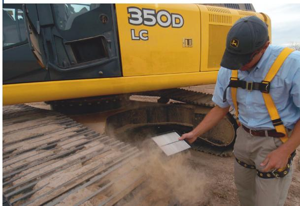
**Andy Nicolas** taps dust out of the 350D's externally mounted cab-air filter. (Note the open door of the compartment just below the cab window.) This filter was positioned inside the C-Series cab, behind the seat, and not as easily serviced.
