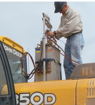
**Above:** Auxiliary tanks used to check fuel consumption during the trenching comparison were fitted with an integral lifting system and a load cell to facilitate weighing and precise measurement.
