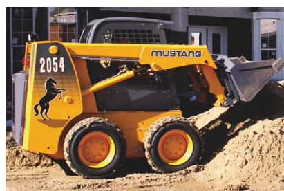
To improve the operator's view, Mustang re-engineered its ROPS/FOPS enclosure for the 2054 (and 2044, in a smaller class) with a larger rear window and redesigned side screen. Hand controls require 18 percent less control effort.
