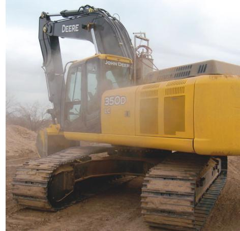
**Brian Ruppert gave us a convincing demonstration of the effectiveness of the 350D's reversing fan. After backfilling trenches in extremely dusty conditions, he activated the system, and we could hear the fan spool down, pause, and then come rapidly up to maximum speed in the opposite direction, blasting out a cloud of dust.**
