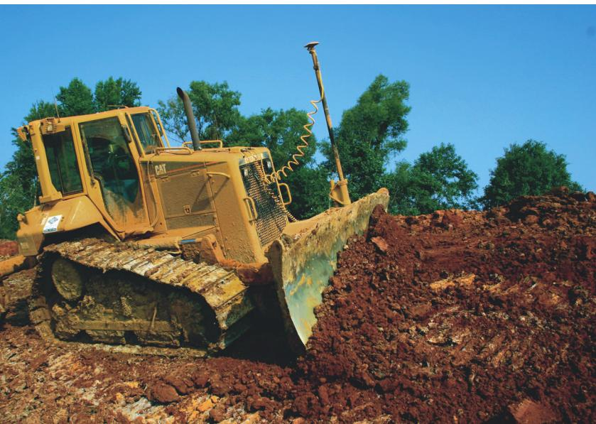
**Stanley Construction has two Cat D6 dozers with GPS grade controls that are making new operators more productive. Al Stanley credits the image on the monitor screen. "The operator . . . sees the slope and how his blade is oriented. He's no longer dependent on his experience to be able to translate what that stake says."**
