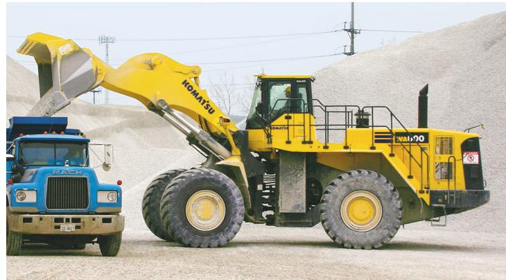
**Raising engine horsepower 12 percent tied Komatsu's WA600-6 at the top of the 375- to 575-hp size class with Volvo's L330E. The new Komatsu is the heaviest loader in its class and has the highest dump clearance and greatest tipping load.**
