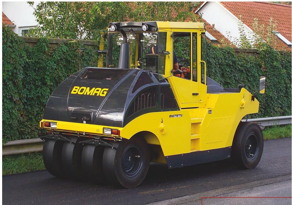
**The operator's station for the BW24RH and BW27RH, available with an optional enclosed cabin, features two steering positions and a sliding/swiveling seat to accommodate operator preferences.**
